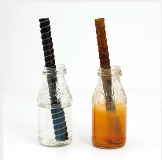
Comparison of KEco Rebar and Steel Rebar Rust
